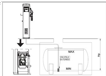
DIAGRAM: FIXING THE UNIT TO THE GROUND
