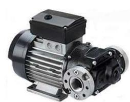
Available in both single and three phase, this mains powered Piusi pump consists of a pump head, motor and have an incorporated bypass valve. This 1" BSP flanged diesel transfer pump is supplied with a simple on/off button, and thanks to its thermal motor overload protection is suitable for continuous running.
