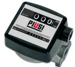
Thanks to its low minimum flow rate the K33 diesel fuel flow meter can perform well in gravity flow conditions as well as in pump installations. This combined with the fact that its face can be rotated to allow the flow from four directions makes this fuel counter meter a flexible solution.
