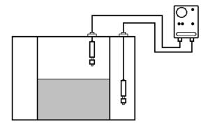
The Bund, Overfill or combined Bund & Overfill Alarms are powered either by a PP3 block 9V battery or the 230V mains supply.
